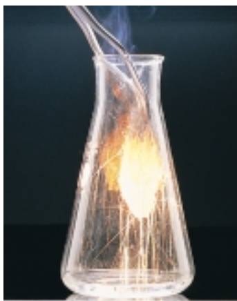
Figure 2.59 Iron combines with pure oxygen in the flask to form iron oxide. This is the same reaction as the rusting of iron, but happens much faster.
