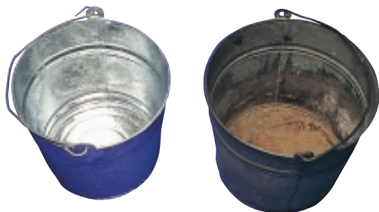
Figure 2.68 The bucket on the left has been galvanized.
