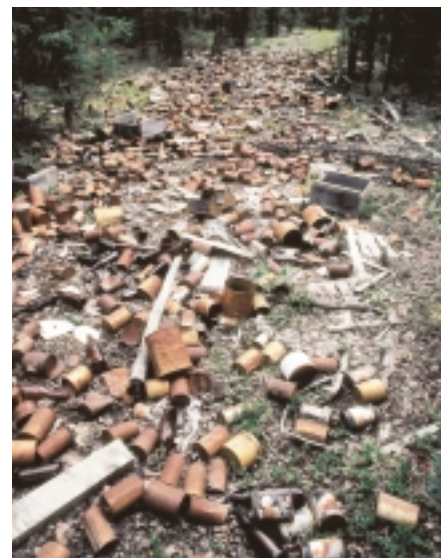
Figure 2.60 The surface of a can that contains iron corrodes quickly outdoors. The rust formed on the surface of the can flakes off easily, so the can continues to corrode. The surface of an aluminum can oxidizes very quickly. The aluminum oxide formed makes a tough protective layer, which does not flake off easily. Therefore, aluminum cans will take over 400 years to degrade. How can you tell that most of the cans in this picture contain iron?
