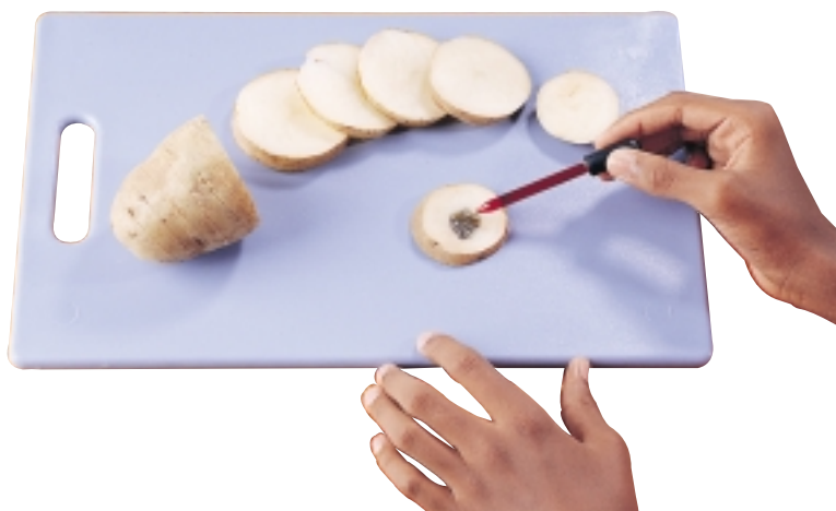
Figure 2.48A When iodine solution is placed on a raw potato, the iodine reacts with the starch to produce a blue-black colour. Colour change can indicate a chemical reaction.
