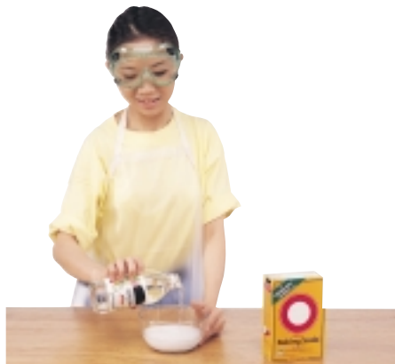
Figure 2.50 When vinegar is poured on baking soda (sodium hydrogen carbonate), bubbles of carbon dioxide gas form quickly. Water and sodium acetate are also formed.
