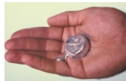
Figure 2.34 The melting point of gallium is so low that it will melt in a person's hand.
