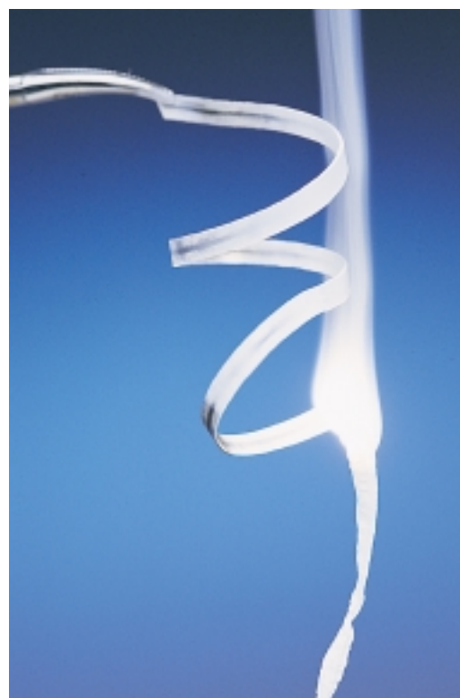
Figure 2.28 When magnesium burns, it gives off intense white light and white smoke. Since magnesium burns in carbon dioxide, what kind of fire extinguisher can be used to put out a magnesium fire?
