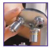
the medium-power lens so that it points at the stage. You should hear a "click" when it is in place. Use the fine adjustment knob to focus the image.
