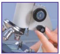
When your slide is in focus, try using the medium-power objective lens. Watch from the side of the microscope.
