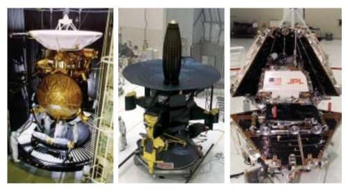
**Figure 3.17** These photographs show the preparation of three different space probes. Each probe must be completely free of contamination, which is why all the workers visible in the photos are wearing specially designed hygienic suits.
