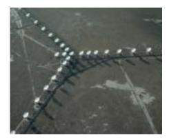
**Figure 3.13** The Very Large Array simulates an antenna with a diameter of hundreds of metres.
