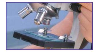
4 Watch the stage from one side of the microscope. Carefully turn the coarse adjustment knob until the lens is as close to the slide as possible without touching it.
