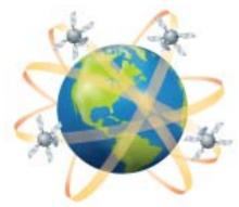
Figure 2.28 With 24 satellites in orbit, there are at least three above the horizon, relative to a person's location on Earth, at any one time.
