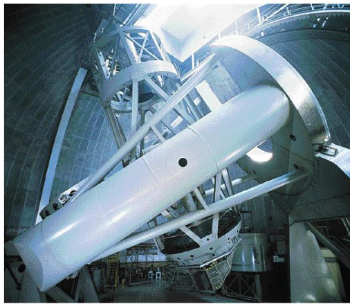
The Hale 200 inch diameter reflector on top of Mount Palomar in California.
