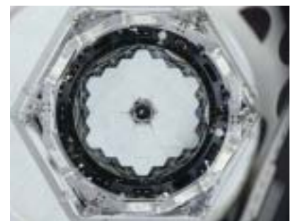
Figure 3.6 One of the Keck Observatory’s two telescopes, showing its 10-m mirror made of 36 hexagonal mirrors
