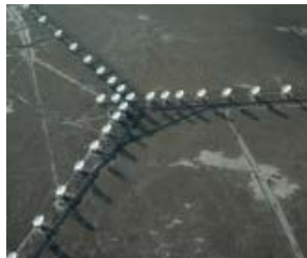
Figure 3.13 The Very Large Array simulates an antenna with a diameter of hundreds of metres.
